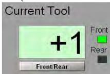
3. Move the Z axis to align the tool to the face of your reference and once aligned click the Z Zero button and the Z DRO will reset to 0. Then click the Touch Z button which puts the current Z DRO value into the tool table.
