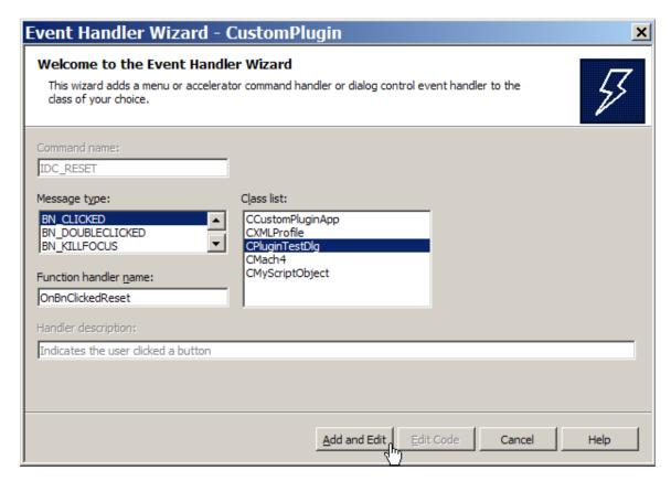
Now you can add the code to make this button perform a "Reset" operation on Mach3. This is done by using the DoButton Intrinsic to push the Mach3 "Reset button".
