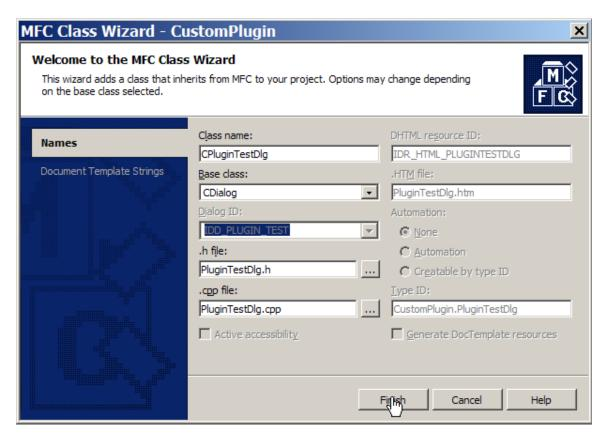
This results in two new files, PluginTestDlg.cpp and PluginTestDlg.h. They will be used to create a modeless dialog.
