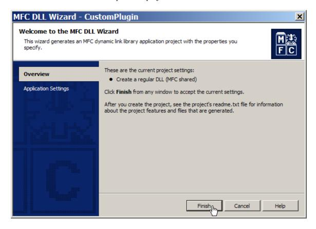
The MFC DLL AppWizard uses a shared MFC DLL which is USUALLY a bad thing, so we will change that to using the MFC static library first. Do this by selecting
