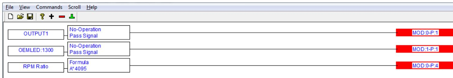
Rung one watches standard Mach OUTPUT1, when it goes ON, the signal is passed to Modbus Local Address “0”, serial Plug-in enabled, Cfg #1.
