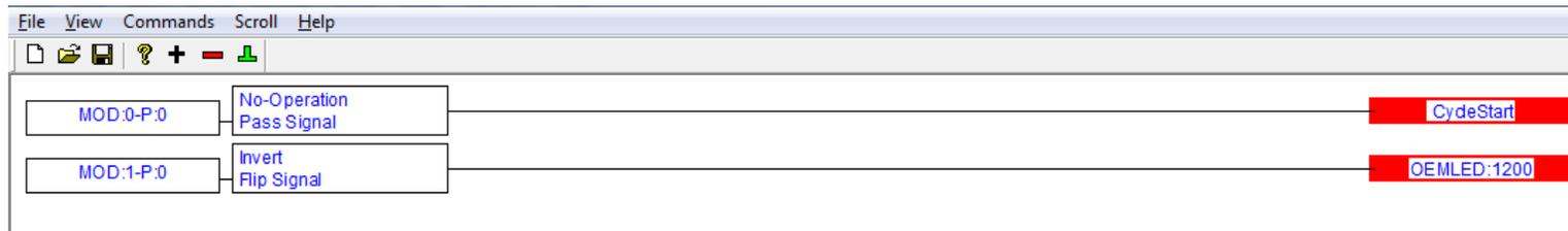
This one shows Inputs from Modbus Local Address “0” (corresponds to hardware address 2000), goes through a No-OP lobe (means it just passes the info straight through, to the Button “Cycle Start” thus you can start your G-code cycle with an external button push. Note the input nomenclature, is “MOD:0-P:0” (means Modbus input since it is on the left side, Local Var Address “0”: P = Plug in Enabled: 0 = Cfg “0”).
