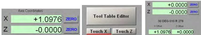
If you open the tool table you will see the X offset for tool #2 and the value shown is absolute based on radius mode.
